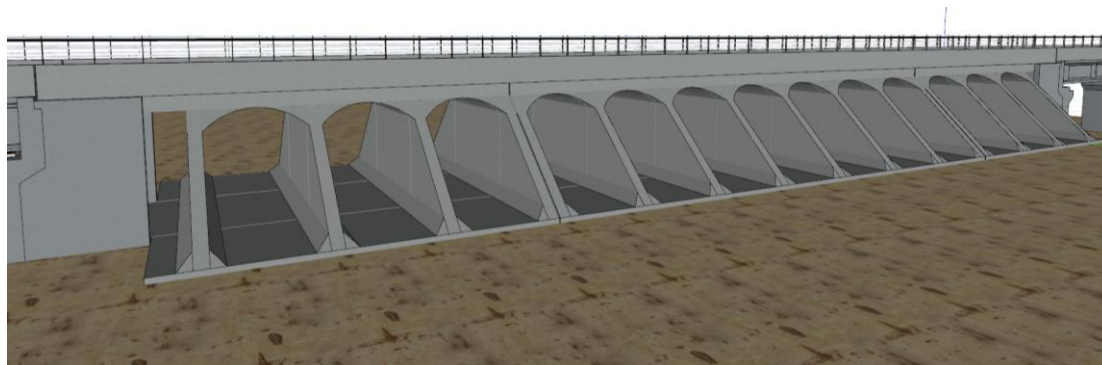
Figure 12. Perspective illustration of box culvert arrangement
