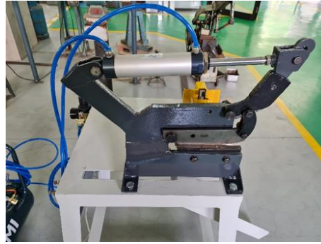
Figure 7. The position of inserting the plate into the cutting knife.
